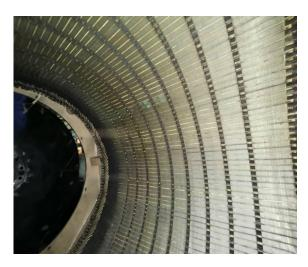
ALTERNATOR INTERNAL CHEMICAL CLEANING ON SITE 3 SETS OF 6L23/30H
